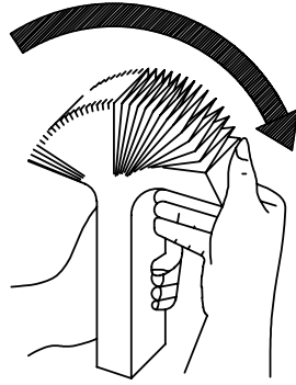
Fig. 5.5 Loosening the Chart Paper
